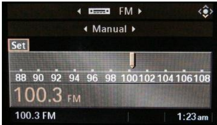
Manual station search in a CCC system
